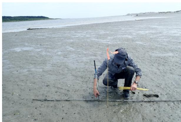
**Measuring sediment depth over buried concrete pavers**
